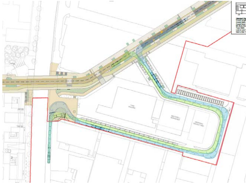
Proposed access works to enable continued access to Arriva bus depot and other occupiers
